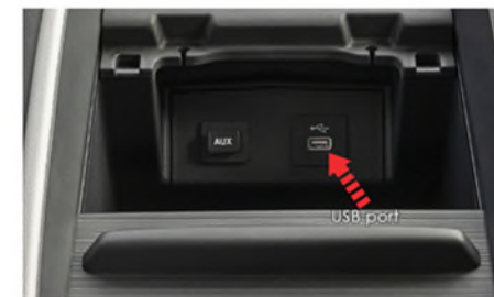
USB data port on Honda Odyssey is located in the center console, slide the cover open to access the port.
