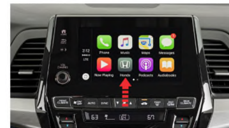
Touching Honda icon on the home screen of CarPlay takes you to the vehicle's infotainment system software - Honda Odyssey fifth generation shown
