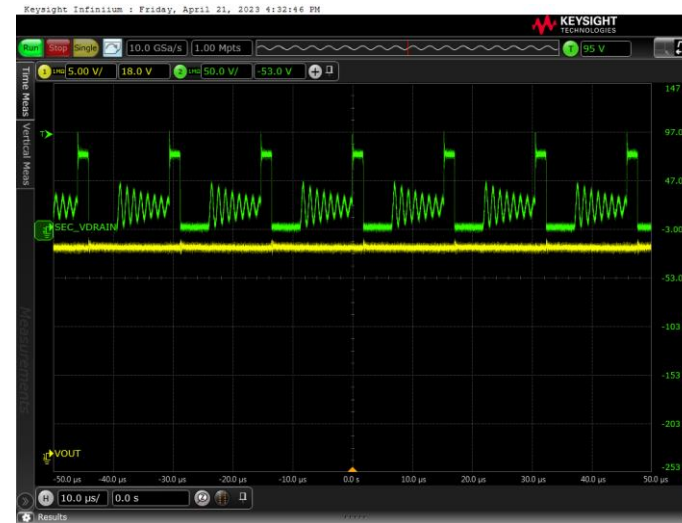
Vout and secondary SW node Steady state
