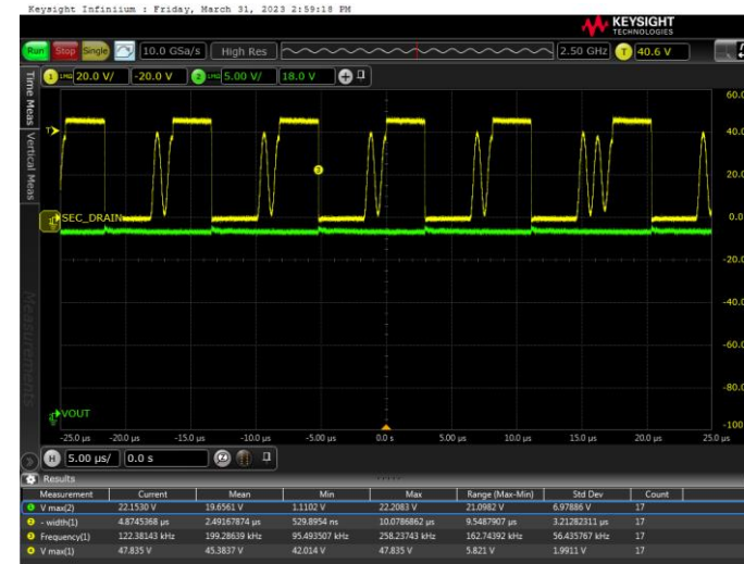
Vout and secondary SW node start up
